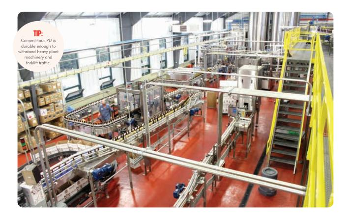
The robust build up of polyurethane avoids floor failures from extreme temperatures and as its thermal coefficient of expansion is similar to that of concrete it will move with the underlying substrate during thermal cycling conditions, avoiding cracks and gaps appearing in the floor's surface.
