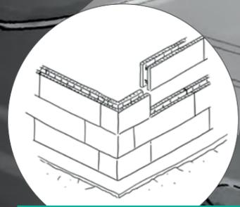
Nudura Insulated Concrete Forms (ICF) for foundations and wall systems are stronger, better insulated and can be installed in much lower temperatures than traditional framing.
